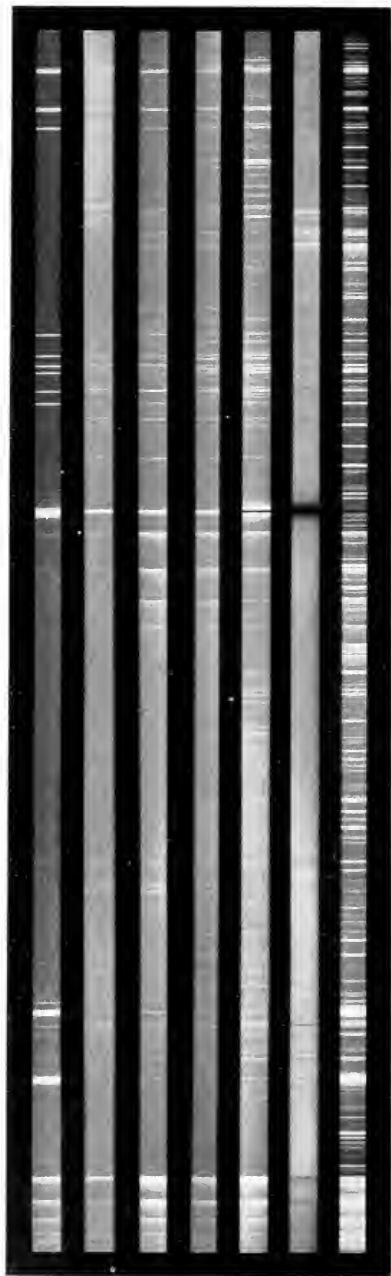
THE SPECTRUM OF CALCIUM IN THE ARC AND IN THE ELECTRIC FURNACE, SHOWING THE EFFECTS OF CHANGING THE TEMPERATURE AND THE QUANTITY OF VAPOR
